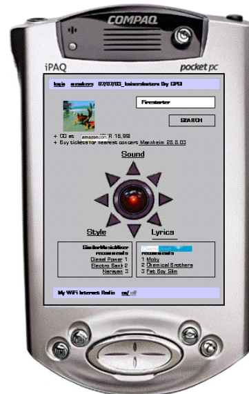
Figure 1. The music assistant consists of a wireless enabled handheld (PDA) and the functionality at server-side can be activated within a standard web browser (e.g. PocketExplorer for PocketPC) supporting flash plugin. The virtual joystick is implemented as a flash animation.
